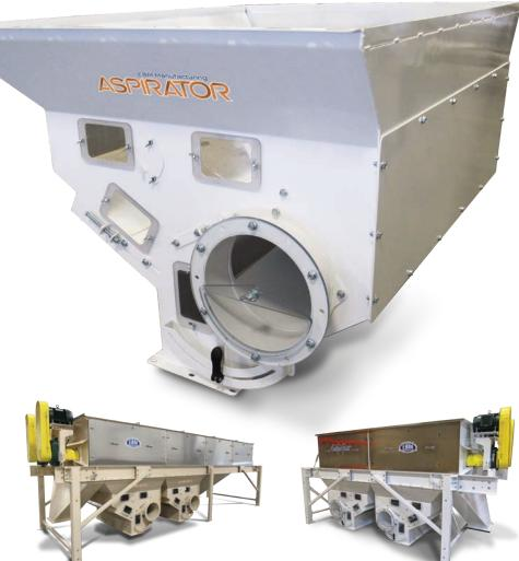
The single-pass, closed-circuit EBM Manufacturing Aspirator utilizes air to remove fines, dust, and lightweight material. It is best suited for small grains including, rice, wheat, barley, and oats, but may be applied to a number of different products. The aspirator can be used after the screening process in conjunction with the Gentle Roll™ screener or as a stand-alone.
